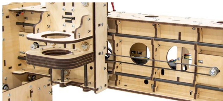
Completed Y Axis Belt Installation
