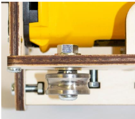
Completed Spindle Mount Assembly (back view):
