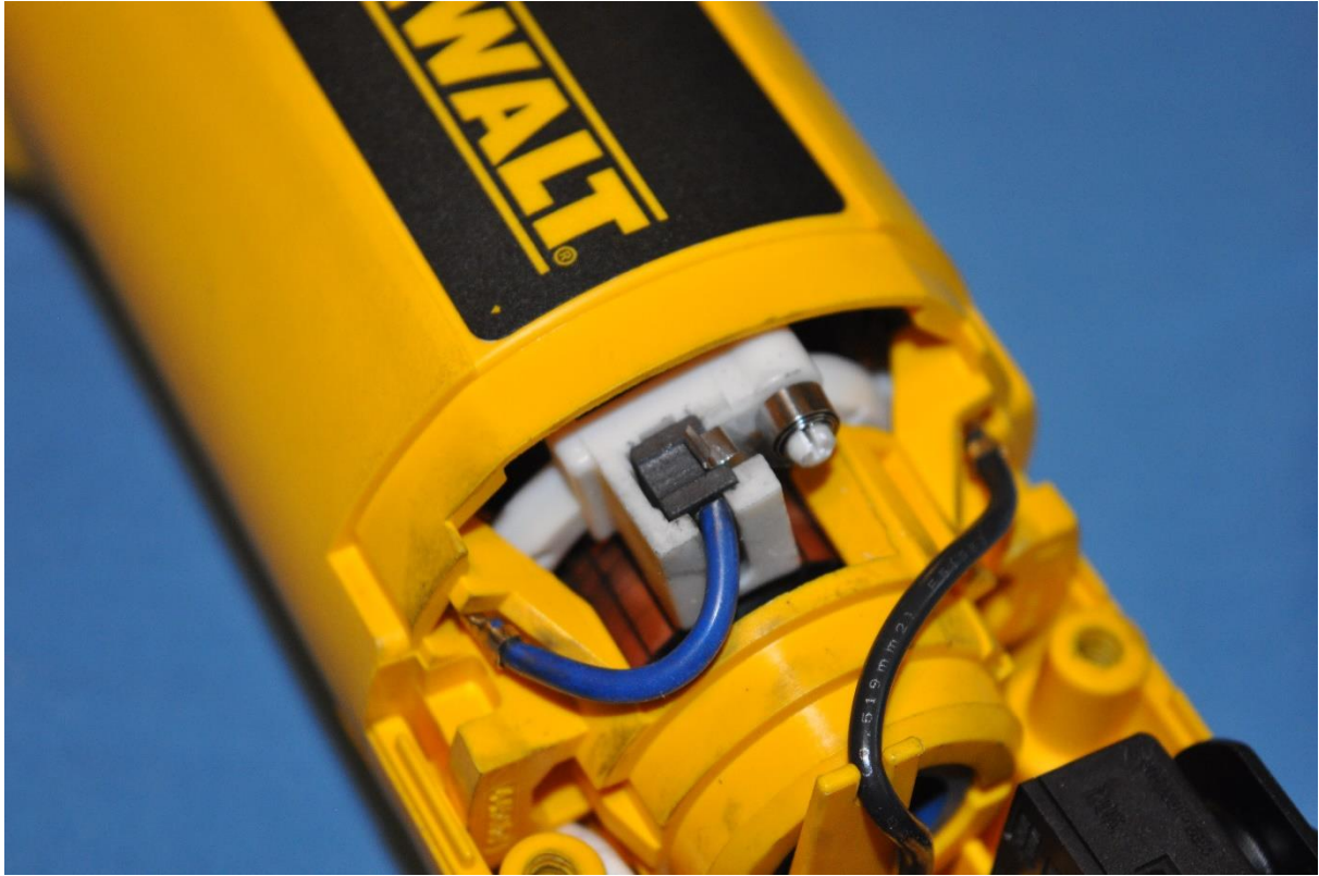
Install the back cover and place components and wires as shown.
