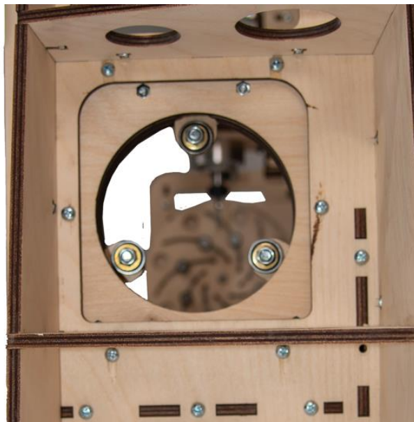
Finished installation of Pass Through Tail Stock, outside view.
