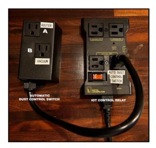
4. When the Router plugged into "A" is energized, the vacuum port "B" will be energized after a couple of seconds.
