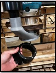
uses less than 8 AMPS. Best to use a 20 AMP circuit. You do not want to blow the breaker while you are carving.
