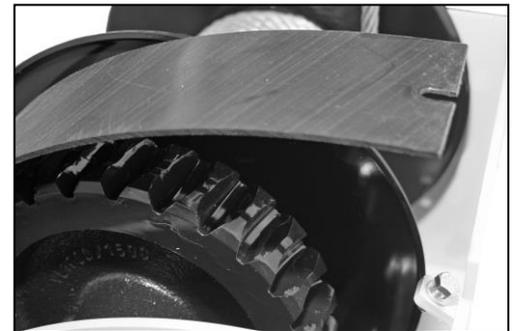
To enable the load pressure brake to function correctly, the winch must carry a minimum load of approx. 5% of the nominal load.
