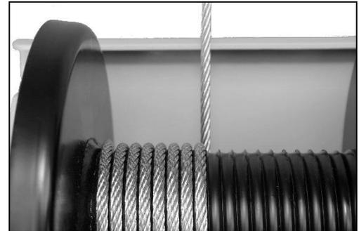
The cable is mounted by means of the fixed cable clamp.
