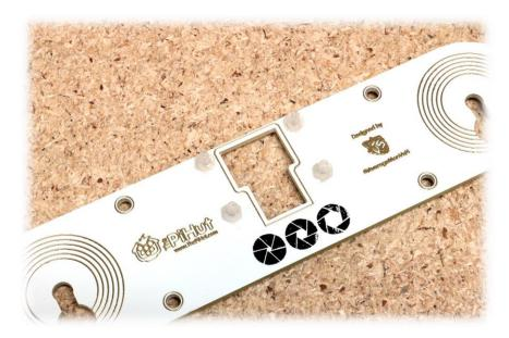
4. Next place your camera module on the rear of the board with the sensor through the large centre hole. The camera's mounting holes should slide on the M2 screws that you fitted.
