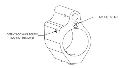
The Gas block is treated with black nitride and compatible with the AR15/AR10 platform, .750 barrel. Please observe the following guidelines:
