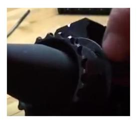
**3.** Clean the threads on the upper receiver, apply lubricant (we recommend graphite free, high temp wheel bearing grease or similar) on barrel nut with jam nut on, and install the new barrel nut until it is firmly tightened by hand.
