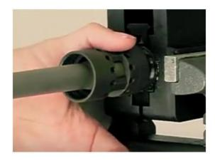
**4.** Tighten the barrel nut to 35 ft.lb. Proceed cautiously to align one of hole in the barrel nut right in the top below the gas tube hole. If when torque applied is over 40
