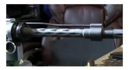
**6.** Slide in the free float quad rail; rotate the rail onto the barrel nut until it makes contact with the jamb nut. Adjust the jam nut to allow the top of rail contact and align with upper receiver rail. Tighten the jam nut. Secure the quad rail with anti-rotation screw.
