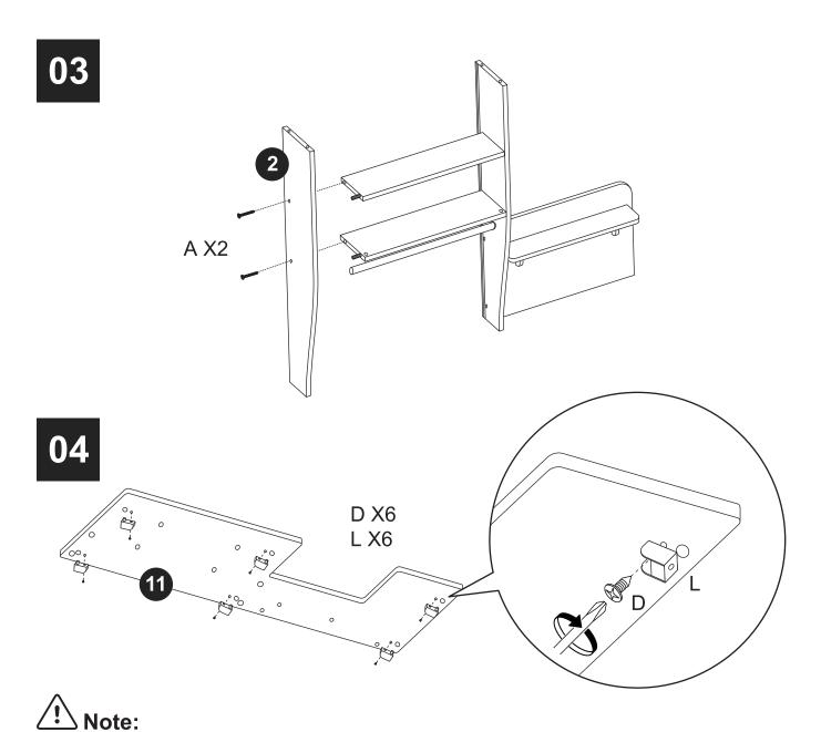
Tighten part **L** manually. Otherwise, an electric screwdriver will damage it.
