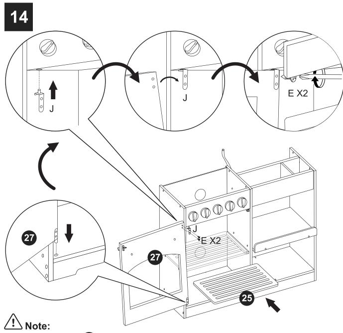
Firstly, insert part **27** into the bottom holes of the base. Then insert part **J** on the top. Align part **J** with the top of part **27** and screw them with two screw **E**.
