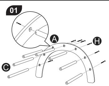
Align and insert the notched end of pole (a) into board (A).
