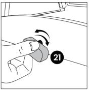
Note: Adjust the tightness of the 21 screw to control the wheel's speed and its ability to stop.
