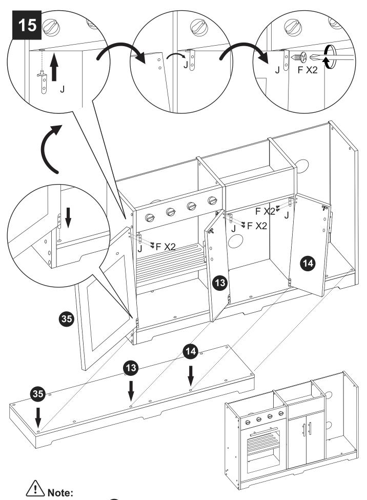
Firstly, insert part 35 into the bottom holes of the base. Then insert part J on the top. Align part J with the top of part 35 and screw them with two screw F. Repeat the above steps to assemble part 13 and part 14.
