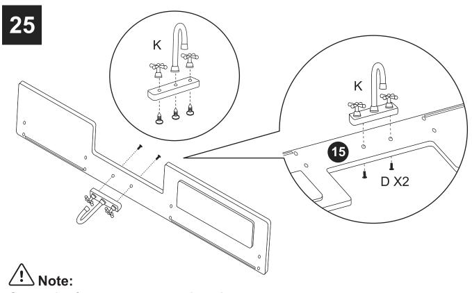
Screw the faucet manually, otherwise, the electric screwdriver will damage it.
