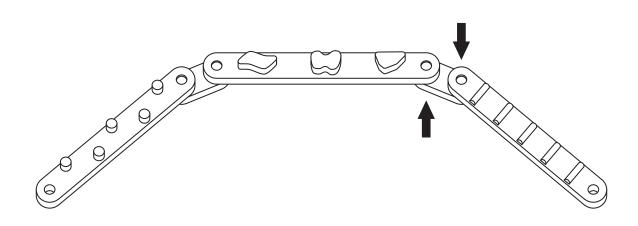
Continue connecting the beams by placing the connector B on both sides of beam A.
