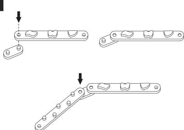
Connect 2 beams A with 1 connector B by pressing the wooden peg on the connector until the beams are firmly secured.
