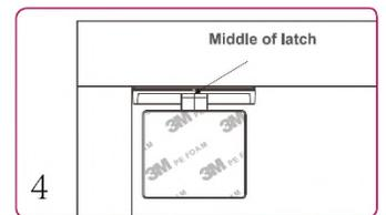
IF YOU ARE NOT USING THE OPTIONAL HARDWARE, ALLOW ADHESIVE TO FULLY CURE FOR 24-HOURS
