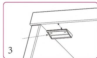
STEP 3(B): CABINET STYLE #2 – Align the catch plate set back equal depth to the thickness of the door of cabinet. See figure 3. Mark with a pencil, peel backing off the adhesive and install in the marked location. Always hold and press firmly for a few seconds while adhesive makes initial bond.
