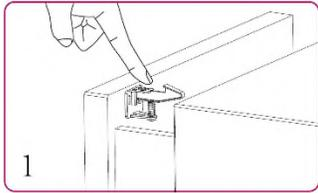
STEP 1: Thoroughly clean all surfaces where locks & catch plates will be installed using rubbing alcohol or a degreasing cleaner. Let the surface completely dry.
