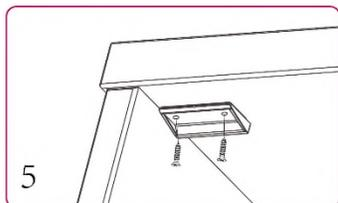
STEP 5: Install optional mounting screws. Drill small pilot holes, 2 per catch plate, and 2 per lock. WARNING – Do not drill pilot hole too far into cabinets as pilot hole may extend through entire cabinet door to outside surface. Once a pilot hole has been drilled, screw in hardware with a Philips head screwdriver. Hand tighten only. Over tightening may cause screw to strip hole in cabinet and may no longer function as a mounting hole.
