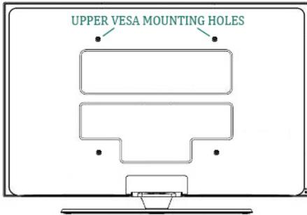
**STEP 1** - Locate the upper VESA mounting holes on the back of TV and select the correct included bolt size (and washer) to fit TV. Note: washers are only required (and included) for the smallest bolt size.
