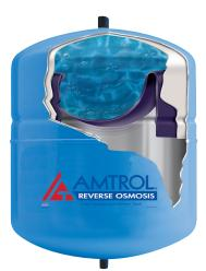
Polypropylene liner and butyl rubber diaphragm are locked together with Amtrol's unique hoop ring and groove design.
