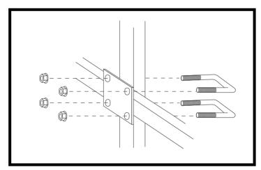
Use UBOLT 3/8-16x2.06x5.25 (for 2" Wide Tubing) to secure Canoe/Kayak Crossbrace Bar to Upright Bar with 3/8-16 Serrated Flange Nuts.
