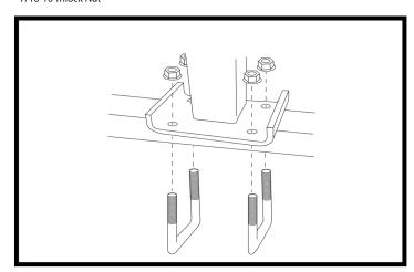
Use UBOLT 3/8-16x2.06x5.25 (for 2" Wide Tubing) or UBOLT 7/16-14x2.06x4.31 (for 1.5" Wide Tubing) to secure Canoe/Kayak Upright Bar to Rear of Trailer with 3/8-16 Serrated Flange Nuts, or 7/16 Trilock Nuts.
