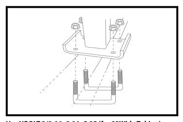
Use UBOLT 3/8-16x2.06x5.25 (for 2"Wide Tubing) or UBOLT 3/8-16x3.06x4.5 (for 3"Wide Tubing) to secure Canoe/Kayak Upright Bar to tongue with 3/8-16 Serrated Flange Nuts.
