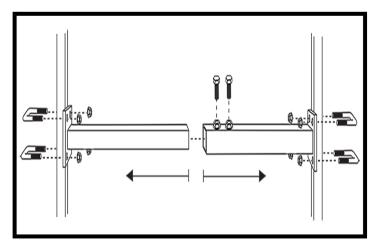
\*\*For mounting optional Galvanized Adjustable Stability Bar only. Use UBOLT 3/8-16x2.06x2.88 to secure backing plate to Upright Bar with 3/8-16 Hex Flange Top Luck Nut. Use Pre-fitted pinch bolts to secure desired length.
