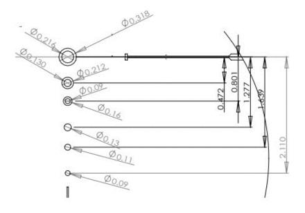
The measurements in the image above are all listed in MOA. These measurements will hold true as long as the FPS dial is set to match the FPS of the crossbow in use.
