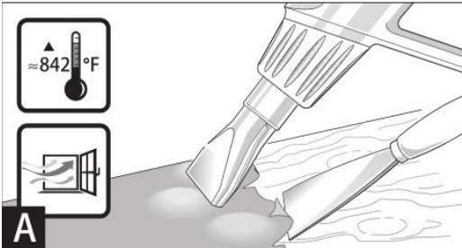
Mount the wide jet nozzle (included). Briefly soften the varnish applying hot air and remove it using a sharp, clean scraper or putty knife. Applying heat too long will burn the varnish, making it more difficult to remove.
