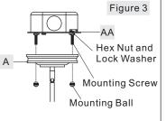
not, adjust the length of the nipple on the Crossbar Assembly (AA) by unscrewing the preassembled hex nut and lock washer and then screwing the mounting screws in or out of the crossbar until the correct length is achieved. Once the Ceiling Canopy (A) is secure, remove the mounting ball and Ceiling Canopy (A) and proceed to Step 4.
