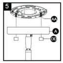
7.Angled mounting recommended for a vaulted or angled ceiling.
