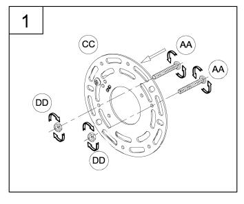
1. Loosely thread the screws (AA) and the hex nuts (DD) onto the round mounting plate (CC). You now need to adjust the screw length according to the fixture canopy depth.
