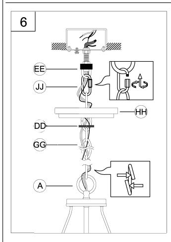
NOTE: During this step, determine the hanging length of your fixture by removing chain links (GG) and optionally cutting the electrical and ground wire to length.
