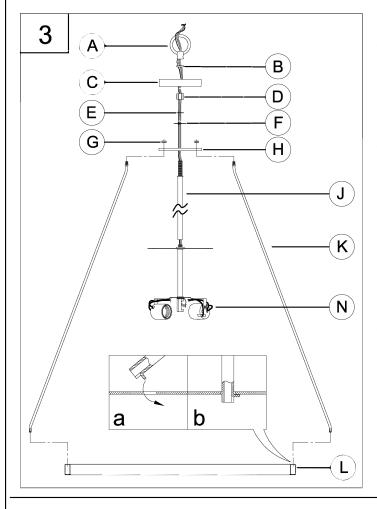
3. Pass the cup (H), flat washer (F) and lock washer (E) onto the stem (J) and use the hex coupling (D) to secure it tightly to the stem (J).
