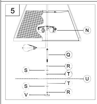
5. Thread the lamps (not included) into the fixture sockets. Use 60-watt MAX incandescent medium base lamp, SBCFL or SBLED.
