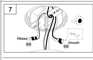
7. Strip 3/8" of insulation from the electrical wire ends. Using wire nuts (BB), connect the RIBBED fixture wire to the WHITE supply wire from the outlet box; connect the SMOOTH fixture wire to the BLACK supply wire. Connect the fixture ground wire and supply ground wire using a wire nut or by fastening to the ground screw on the mounting strap. Push all wire connections into the outlet box.
