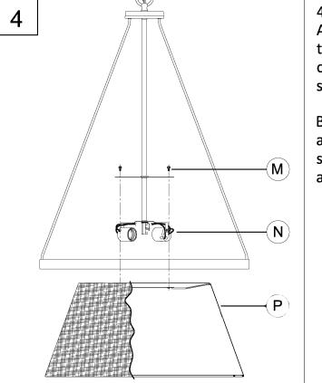
4. Raise the fabric shade (P) up into the fixture (N). Align the 3 holes in the fabric shade top plate with the 3 threaded holes on the top of the socket cluster (N). Use the 3 knurled ball studs (M) to secure the fabric shade (P) to the fixture tightly.
