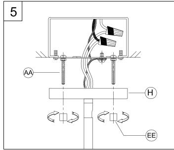
5. Pass the screws (AA) through the two holes in the canopy (H). Secure the fixture to the screws (AA) using the two cylinder nuts (EE). Tighten securely.
