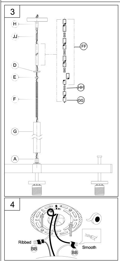
NOTE: During this step, determine the hanging length of your fixture by adding or removing pipes (FF)(GG). The electrical and ground wire may also optionally be cut to length.
