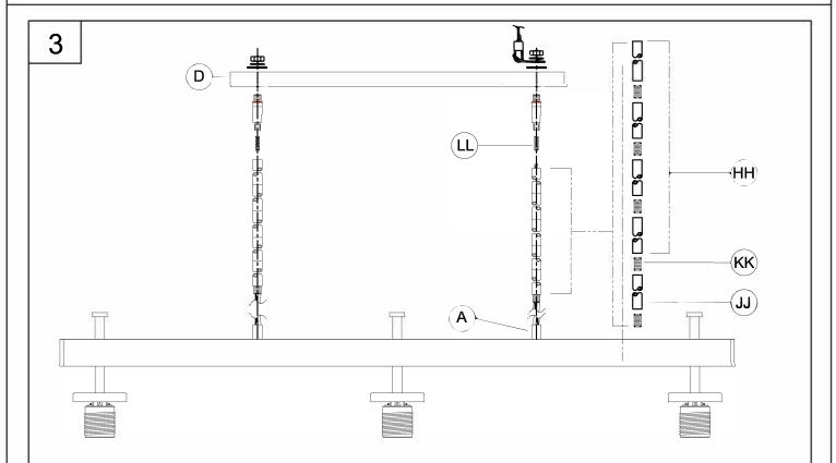
NOTE: During this step, determine the hanging length of your fixture by adding or removing pipes. The electrical and ground wire may also optionally be cut to length. Remove the swivels if they are already assembled to the canopy. You will re-assemble them onto the top of the last pipe before wiring has been passed through during this step. Align them so they will swivel in the same direction.
