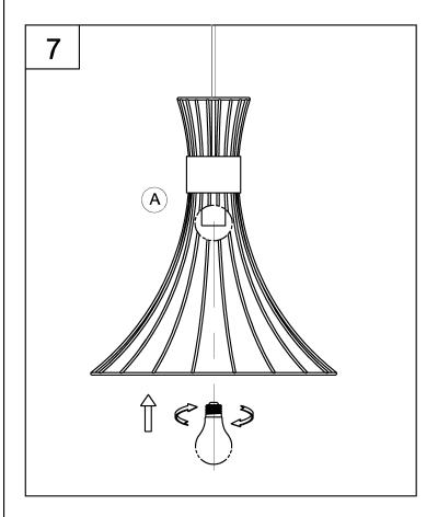
7. Thread the lamp (not included) into the fixture socket. Use 60-watt MAX incandescent medium base lamp, SBCFL or SBLED.
