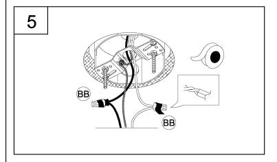
5. Strip 3/8" of insulation from the electrical wire ends. Using wire nuts (BB), connect WHITE fixture wire to the WHITE supply wire from the outlet box; connect the BLACK fixture wire to the BLACK supply wire.
