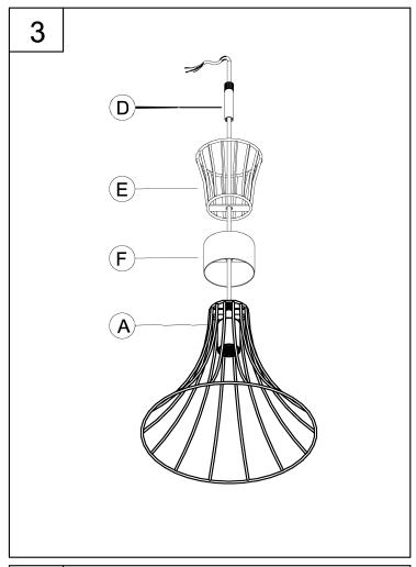
3. Pass the cord from the bottom wire frame (A) through the collar (F) and top wire frame (E) and knurled tube (D). Thread the knurled tube (D) onto the bottom wire frame (A). Tighten the parts securely together (A,F,E) with the knurled tube (D).
