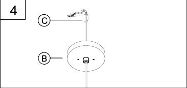
NOTE: During this step, determine the hanging length of your fixture by adjusting the cord length.
