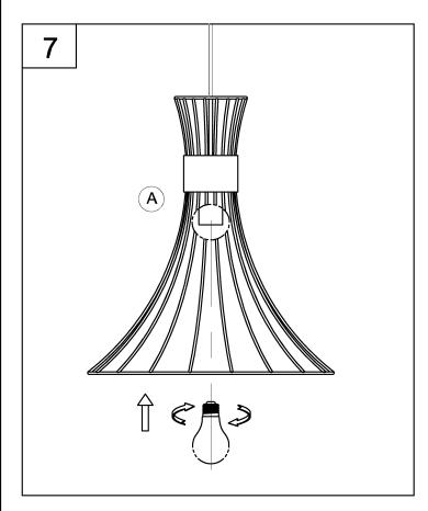
7. Thread the lamp (not included) into the fixture socket. Use 60-watt MAX incandescent medium base lamp, SBCFL or SBLED.
