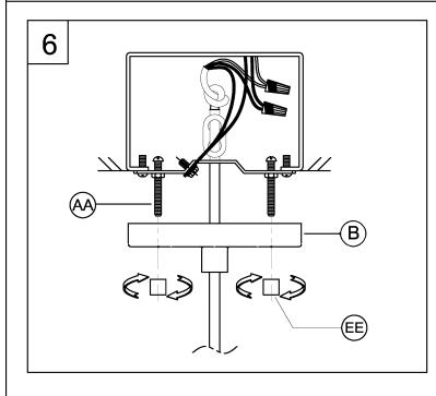
6. Pass the screws (BB) through the two holes in the canopy (B). Secure the fixture (A) to the screws (AA) using the two cylinder nuts (EE). Tighten securely.
