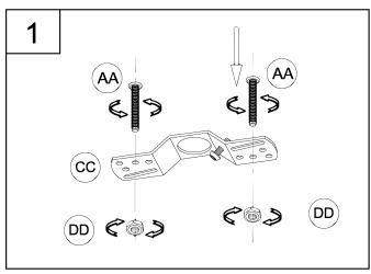
1. Loosely thread the screws (AA) and the hex nuts (DD) onto the swivel mounting strap (CC) as shown. You now need to adjust the screw length according to the fixture canopy depth.
