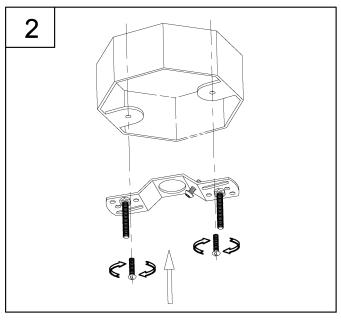
Next, take the canopy down and go back and tighten the hex nuts (DD) up against the mounting strap (CC). You now should have the correct length of threads for mounting the fixture.
