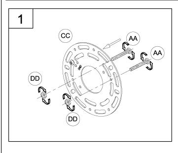
1. Loosely thread the screws (AA) and the hex nuts (DD) onto the round mounting plate (CC).
