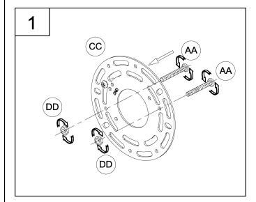
1. Loosely thread the screws (AA) and the hex nuts (DD) onto the round mounting plate (CC).
