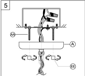
5. Pass the screws through the two holes in the canopy. Secure the fixture (A) to the screws (AA) using the two cylinder nuts (EE). Tighten securely.
