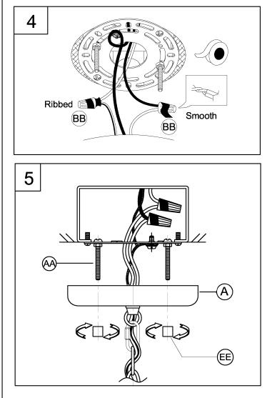
4. Strip 3/8" of insulation from the electrical wire ends. Using wire nuts (BB), connect RIBBED fixture wire to the WHITE supply wire from the outlet box; connect the SMOOTH fixture wire to the BLACK supply wire.
