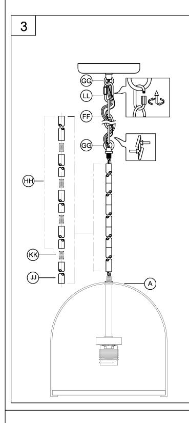
NOTE: During this step, determine the hanging length of your fixture by adding or removing stems and chain links. The electrical and ground wire may also optionally be cut to length.
