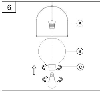
6. Attach the glass shade (B) to the fixture (A) using the socket ring (C) to secure it tightly.
