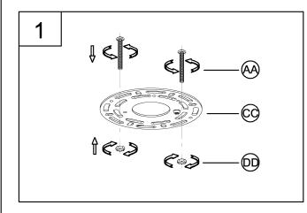
1. Loosely thread the screws (AA) and the hex nuts (DD) onto the round mounting plate (CC) as shown. You now need to adjust the screw length according to the fixture canopy depth.
