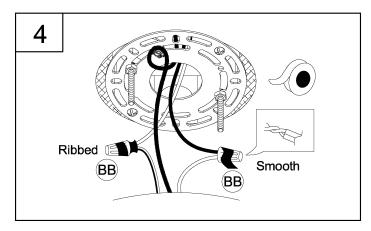
4. Strip 3/8" of insulation from the electrical wire ends. Using wire nuts (BB), connect RIBBED fixture wire to the WHITE supply wire from the outlet box; connect the SMOOTH fixture wire to the BLACK supply wire.
