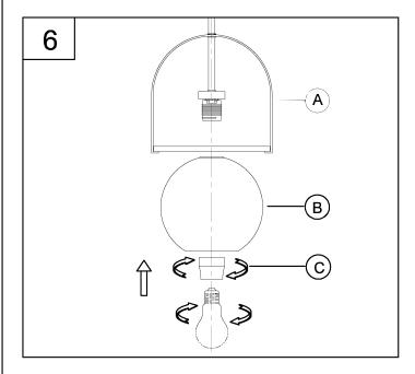
6. Attach the glass shade (B) to the fixture (A) using the socket ring (C) to secure it tightly.
