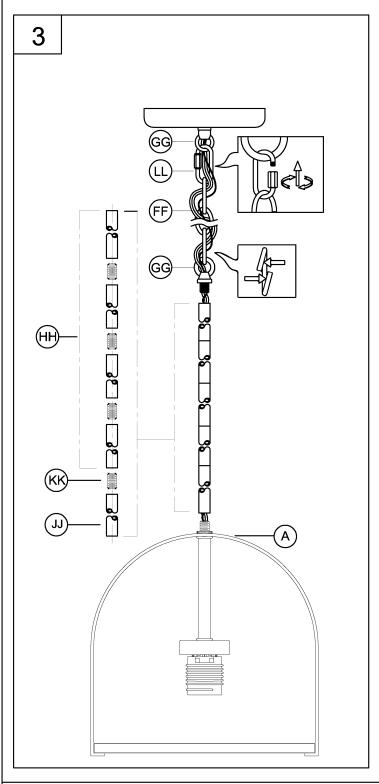
NOTE: During this step, determine the hanging length of your fixture by adding or removing stems and chain links. The electrical and ground wire may also optionally be cut to length.
