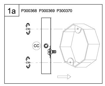
1a. Attach the metal back plate (CC) onto the outlet box using the mounting screws supplied with the outlet box (not provided). Adjust it so it is parallel with the ceiling or wall surface. Tighten securely.
