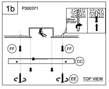
1b. Line up mounting holes on the back plate (CC) with screw holes on the outlet box.
