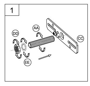
1. Loosely thread the nipple (AA), lock washer (EE) and the hex nut (DD) onto the mounting strap (CC).
