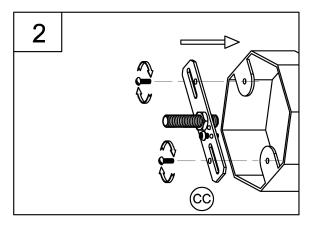
2. Attach this assembly to the outlet box using the mounting screws supplied with the outlet box (not provided). Tighten securely.
