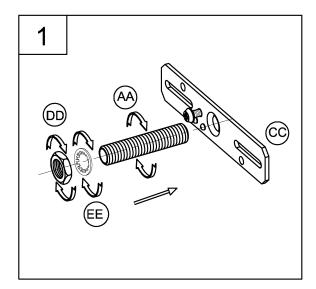
1. Loosely thread the nipple (AA), lock washer (EE) and the hex nut (DD) onto the mounting strap (CC).
