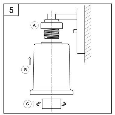
6. Thread the lamps (not included) into the fixture sockets. Use 60-watt MAX incandescent medium base lamp, SBCFL or SBLED.
