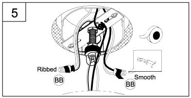
5. Strip 3/8" of insulation from the electrical wire ends. Using wire nuts (BB), connect the RIBBED fixture wire to the WHITE supply wire from the outlet box; connect the SMOOTH fixture wire to the BLACK supply wire
