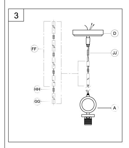
NOTE:During this step, determine the hanging length of your fixture by adding or removing stems. The electrical and ground wire may also optionally be cut to length.
