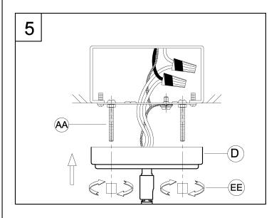
5. Pass the screws through the two holes in the canopy (D). Secure the fixture (A) to the screws (AA) using the two cylinder nuts (EE). Tighten securely.
