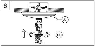
6. Tuck the wires into the junction box and slip the canopy (JJ) over the chain holder. Thread the screw collar (DD) onto the chain holder to secure the canopy tightly to the ceiling.
