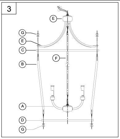
3. Pass the wires from fixture (A) through the stem (F) and body (E). Thread the stem (F) onto the fixture (A)Thread the body (E) onto the stem (F). Secure all parts tightly together.
