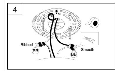
4. Strip 3/8" of insulation from the electrical wire ends. Using wire nuts (BB), connect RIBBED fixture wire to the WHITE supply wire from the outlet box; connect the SMOOTH fixture wire to the BLACK supply wire.
