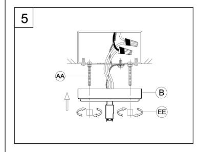
5. Pass the screws through the two holes in the canopy (B). Secure the fixture (A) to the screws (AA) using the two cylinder nuts (EE). Tighten securely.
