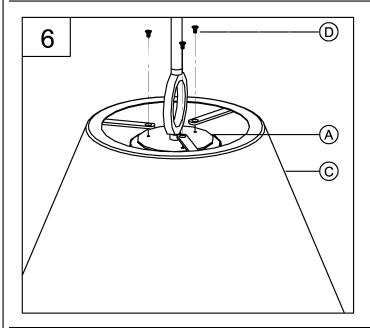
6. Screw the fixture (A) into the metal shade (C) with flat head screws (D). Tighten the parts securely together (A,C) with the flat head screws (D).
