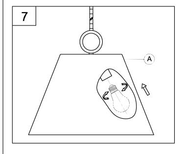
7. Thread the lamp (not included) into the fixture socket. Use 60-watt MAX incandescent medium base lamp, SBCFL or SBLED.
