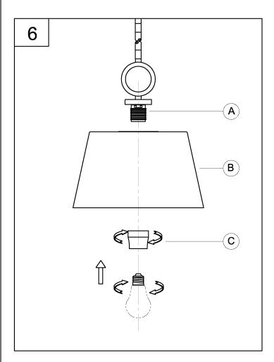
6. Attach the metal shade (B) to the fixture (A) using the socket ring (C) to secure it tightly.
