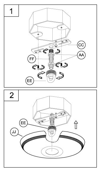
1. Install the chain holder (EE) onto the nipple (FF). Next, loosely thread the hex nuts (AA) onto the nipple (FF) and then thread this assembly onto the mounting plate (CC). Install this assembly to the outlet box using the mounting screws supplied with the outlet box (not included).
