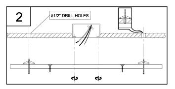
2. Line up the holes in the back plate (BB) with the holes in the junction box. Use a pencil to mark the locations of the two mounting holes. Remove the back plate from the wall.
