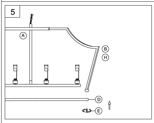
5. Attach the frame (D) to the square arm (B) and square arm (H) using the screws (E) to secure it tightly.
