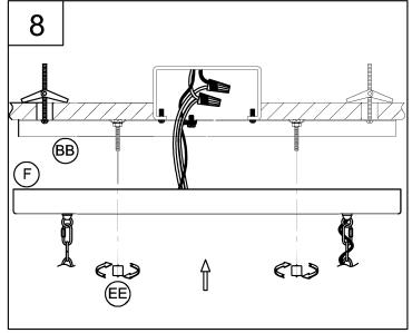
8. Pass the back plate screws (BB) through the two holes in the canopy (F). Secure the fixture (A) to the screws using the two cylinder nuts (EE). Tighten securely.
