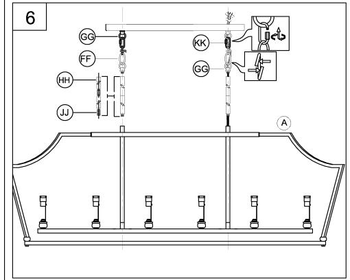
NOTE: During this step, determine the hanging length of your fixture by adding or removing stems and chain links. The electrical and ground wire may also optionally be cut to length.
