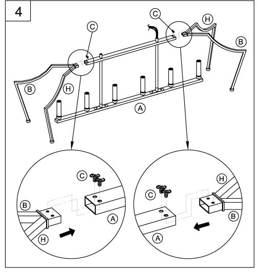
4. Attach the square arm assembly (H, B) to Fixture (A) using the screws (C) to secure it tightly together.
