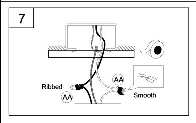
7. Strip 3/8" of insulation from the electrical wire ends. Using wire nuts (AA), connect RIBBED fixture wire to the WHITE supply wire from the outlet box; connect the SMOOTH fixture wire to the BLACK supply wire.
