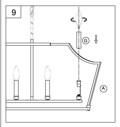
9. Place the candle tube (G) onto the fixture sockets.
