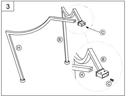
3. Attach the unassembled square arm (H) to square arm assembly (B) using the screw (C) to secure it tightly.
