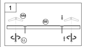
1. Loosely thread the screws (LL) and the toggles (MM) onto the back plate (BB).
