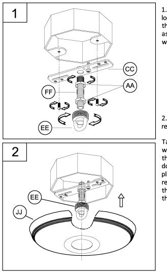
1. Install the chain holder (EE) onto the nipple (FF). Next, loosely thread the hex nuts (AA) onto the nipple (FF) and then thread this assembly onto the mounting plate (CC). Install this assembly to the outlet box using the mounting screws supplied with the outlet box (not included).
