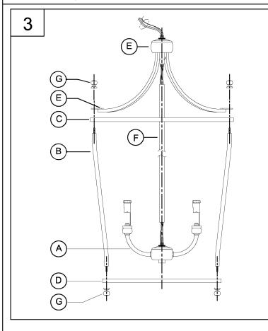
3. Pass the wires from fixture (A) through the stem (F) and body (E). Thread the stem (F) onto the fixture (A)Thread the body (E) onto the stem (F). Secure all parts tightly together.
